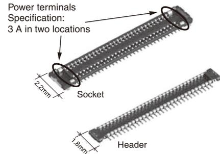
Example; Charging current: Max. 3.0 A (0.3 A/pin, Pitch: 0.35 mm)
