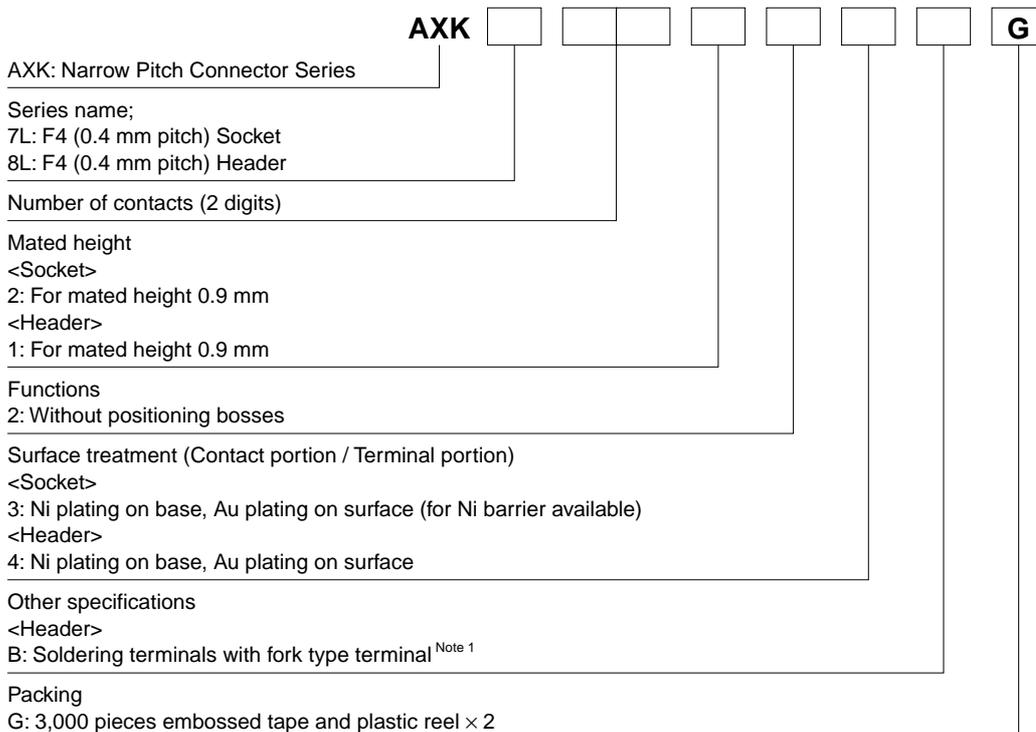
Notes: 1. "B" in the 11th digit of the header part number signifies a fork type soldering terminals to lessen the constraint on amount of solder when mounting, and a construction that makes it difficult when mounting for excess solder to interfere with the socket. Although compatible with the previous parts, these parts are not compatible with the recommended PC board pattern and recommended metal mask pattern.
