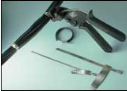
Hand Operated Tool. Installer controlled tension and cut-off.
