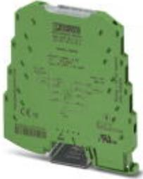
MCR 3-way isolating amplifier, for electrical isolation of analog signals, with spring-cage connection, input signal: 4 mA ... 20 mA, output signal: 0 V ... 10 V
