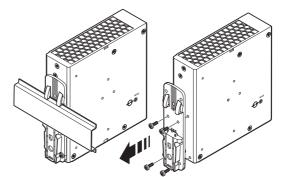
Figure 10 Disassembling the universal DIN rail adapter
