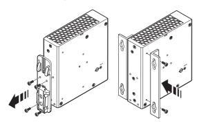
Figure 13 Mounting the UWA 130 universal wall adapter
