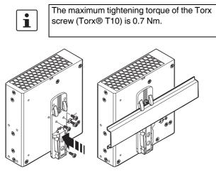
Figure 11 Mounting the universal DIN rail adapter
