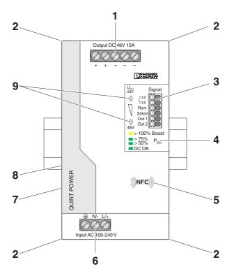
Figure 3 Operating and indication elements
