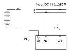
Figure 19 Pin assignment for DC supply voltage
