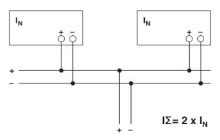
Figure 36 Schematic diagram of increased performance
