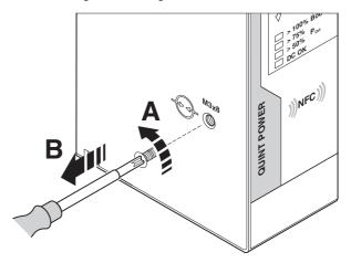
Figure 2 Disconnect gas-filled surge arrester
