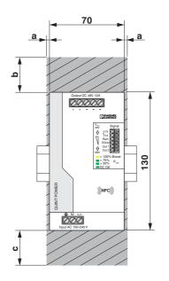
Figure 6 Device dimensions and maximum keep-out areas (in mm)
