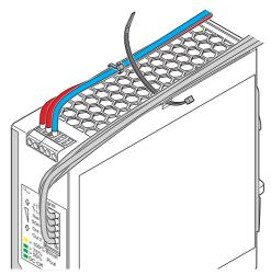
Figure 14 Lay and align connection wiring
