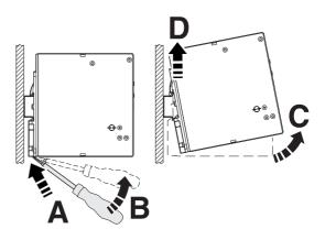
Figure 9 Removing the power supply from the DIN rail
