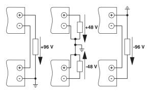
Figure 33 Schematic diagrams in series operation
