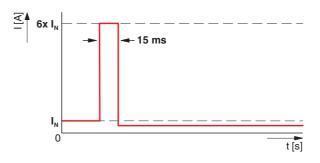
Figure 25 SFB pulse trips circuit breakers
