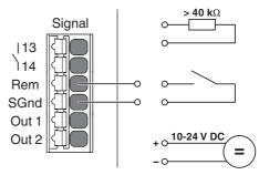
Figure 29 External wiring versions, disable SLEEP MODE
