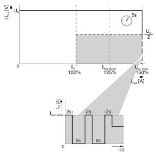
Figure 21 Smart HICCUP output characteristic curve
