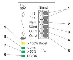
Figure 27 Position of signaling elements
