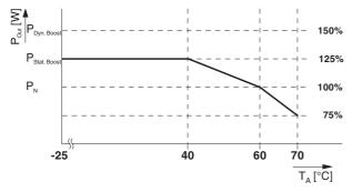
Figure 37 Output power depending on the ambient temperature
