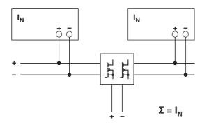
Figure 35 Schematic diagram, redundant operation with QUINT ORING
