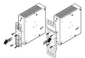
Figure 12 Mounting the UWA 182/52 universal wall adapter
