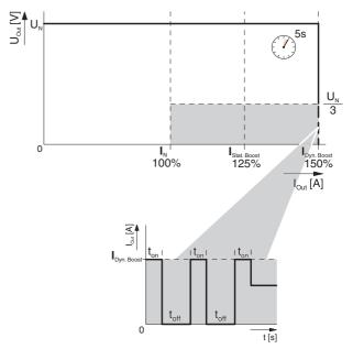
Figure 20 U/I Advanced output characteristic curve
