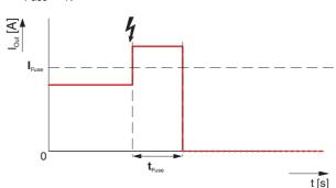
Figure 22 FUSE MODE output characteristic curve
