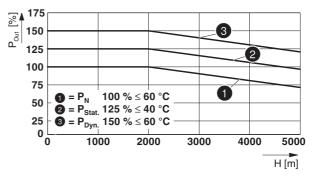
Figure 38 Output power depending on the installation height
