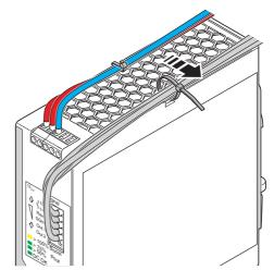
Figure 15 Secure connection wiring with cable binder
