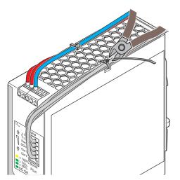
Figure 16 Shorten protruding ends of the cable binder
