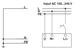
Figure 18 Pin assignment for AC supply voltage
