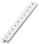
Marker for terminal blocks, Strip, white, labeled, can be labeled with: CMS-P1-PLOTTER, Horizontal: L1, L2, L3, N, PE, L1, L2, L3, N, PE, mounting type: snap into tall marker groove, for terminal block width: 10.2 mm, lettering field size: 10.15 x 10.5 mm
