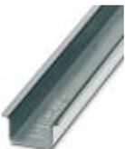
DIN rail, unperforated, Standard profile, width: 35 mm, height: 15 mm, similar to EN 60715: 2001, material: Steel, Galvanized, white passivated, length: 2000 mm, color: white
