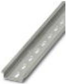
DIN rail perforated, Standard profile, width: 35 mm, height: 7.5 mm, in acc. with EN 60715: 2001, material: Steel, galvanized, passivated with a thick layer, length: 2000 mm, color: silver
