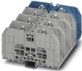
Bolt connection terminal block, nom. voltage: 1000 V, nominal current: 309 A, connection method: Bolt connection, number of connections: 8, number of positions: 4, width: 164 mm, color: gray/blue, mounting type: NS 35/7,5, NS 35/15, direct screw connection
