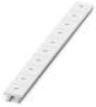
Zack marker strip, Strip, white, labeled, can be labeled with: CMS-P1-PLOTTER, printed horizontally: Identical numbers 1 or 2, etc. up to 100, mounting type: snap into tall marker groove, for terminal block width: 10.2 mm, lettering field size: 10.15 x 10.5 mm
