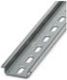
DIN rail perforated, Standard profile, width: 35 mm, height: 7.5 mm, in acc. with EN 60715: 2001, material: Steel, galvanized, length: 2000 mm, color: silver
