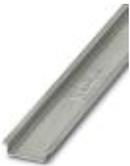
DIN rail, unperforated, Standard profile, width: 35 mm, height: 7.5 mm, in acc. with EN 60715: 2001, material: Steel, galvanized, passivated with a thick layer, length: 2000 mm, color: silver
