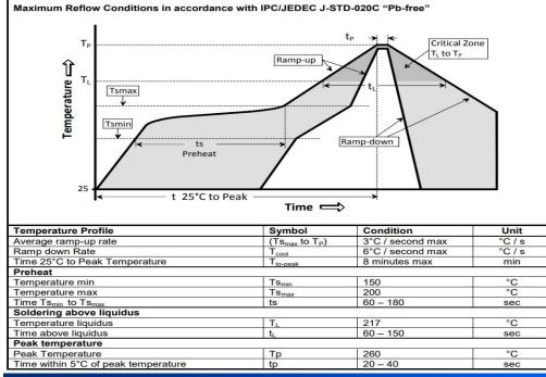
The part may be reflowed 2 times without degradation (typical for lead free processing).
