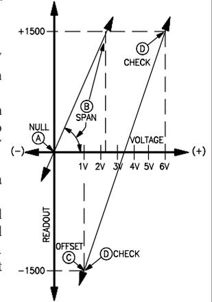
**Example 2 (Positive Offset):** An APLPV is to be calibrated to match a flow transducer whose output is 0 V @ 40 GPM and 5 V @ 650 GPM.
