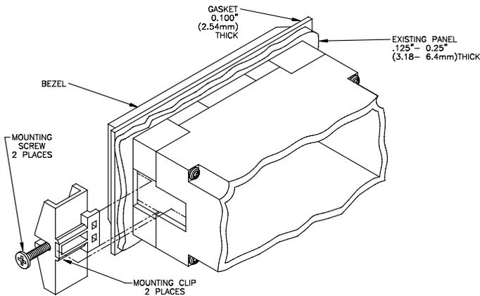
The Apollo Process Voltmeter is designed to be panel-mounted with a gasket to provide a water-tight seal. Two mounting clips and screws are provided for easy installation. Consideration should be given to the thickness of the panel. A panel which is too thin may distort and not provide a water-tight seal. (Recommended minimum panel thickness is 1/8".)
