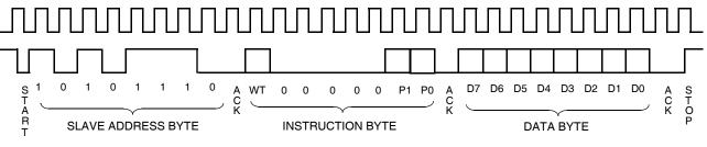
Figure 9. DCP Write Command Sequence
