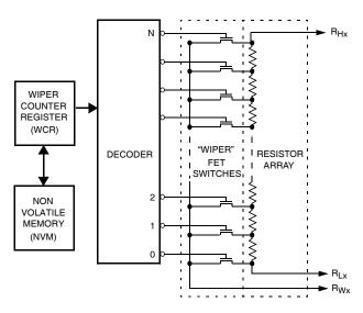
Figure 6. DCP Internal Structure
