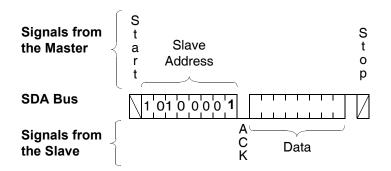
Figure 14. Current EEPROM Address Read Sequence
