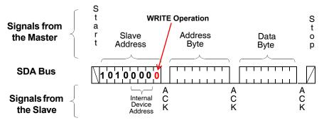
Figure 12. EEPROM Byte Write Sequence
