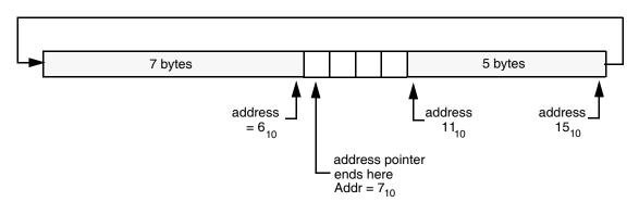
Figure 13. Example: Writing 12 bytes to a 16-byte page starting at location 11.
