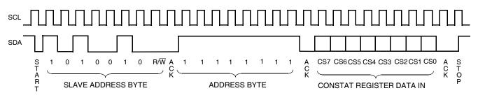
Figure 18. CONSTAT Register Write Command Sequence
