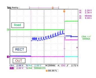
Figure 6. Startup Waveform ( $R_{SET}$ =27k  $\Omega$ )
