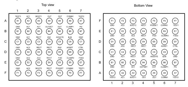
Figure 7. Pin configuration
