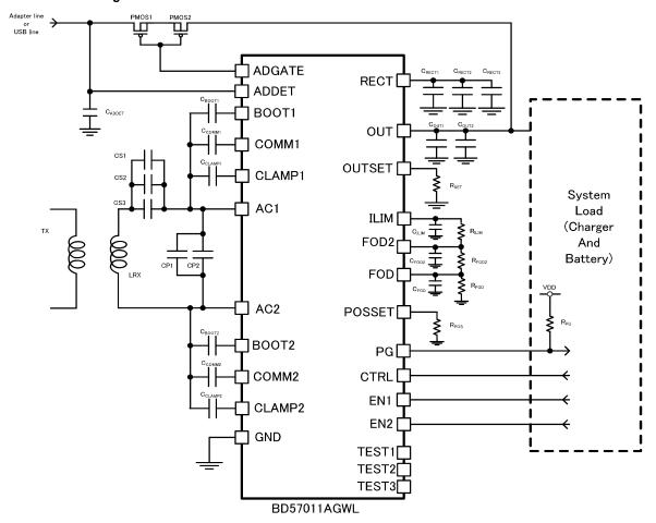
Figure 13. Typical application circuit
