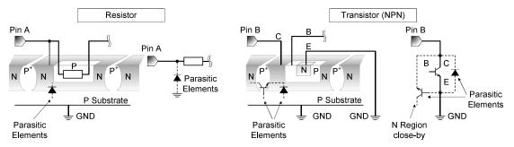
Figure 16. Example of monolithic IC structure
