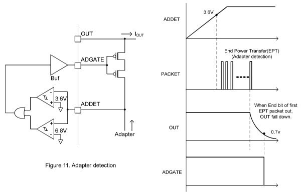
If set to ADDET≥6.8V, it will be in an OVP detection state and will carry out the instant stop of the PMOS of a power path regardless of the existence of wireless power supply.
