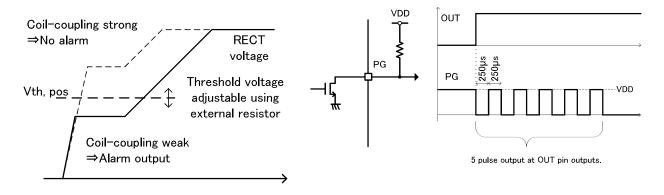
Figure 12. Position Gap alarm
