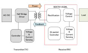
Figure 2. Product position in Wireless Power Supply System
