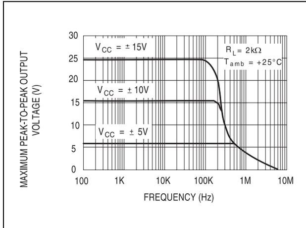
**Figure 3. Maximum peak-to-peak output voltage versus frequency**
