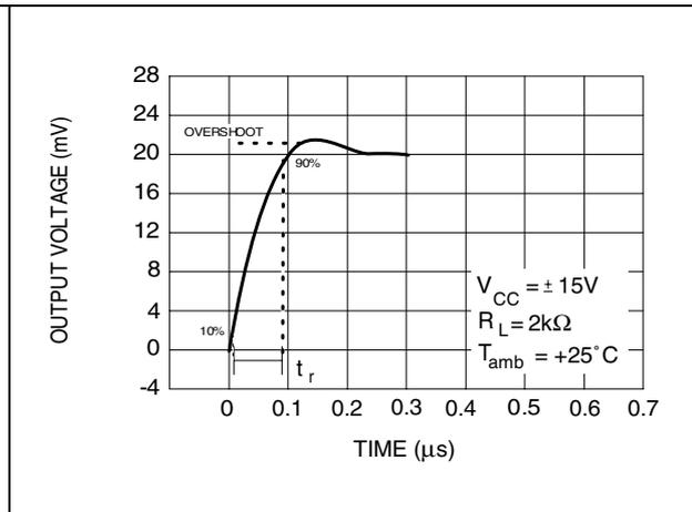
Figure 16. Voltage follower large signal pulse response
