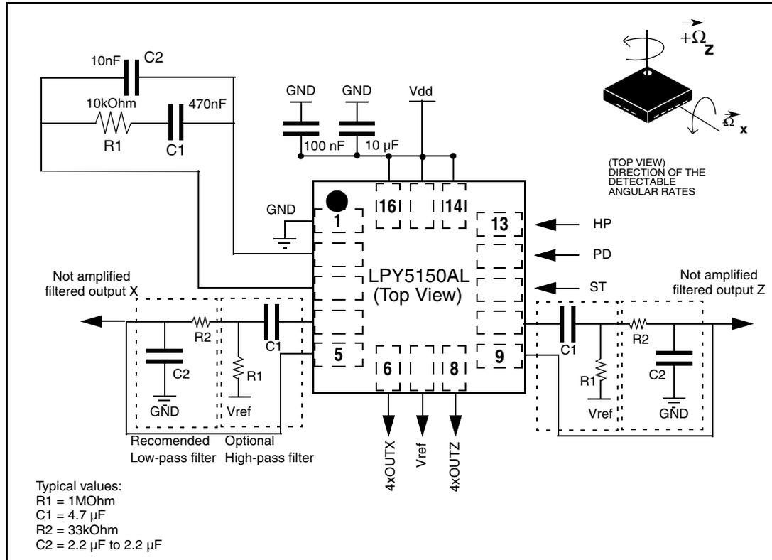
Power supply decoupling capacitors (100 nF ceramic or polyester + 10 µF aluminum) should be placed as near as possible to the device (common design practice).
