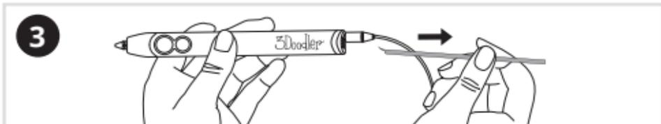
Once the **Plastic** stops reversing, it is safe to remove it from the **Pen** by gently pulling on the back of the strand.
