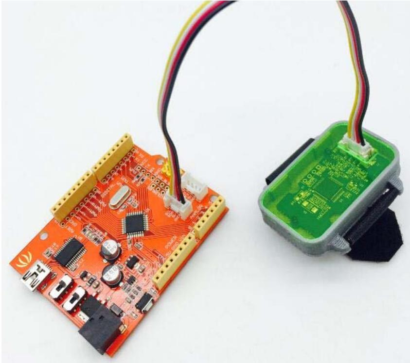
When using the band to fix this module on your finger or wrist, please keep the sensor area contact the skin well and keep no motion, just like the picture.
