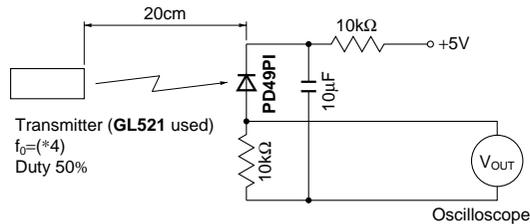
In the above figure, the transmitter should be set so that the output  $V_{OUT(P.P)}$  can be 40mV.
