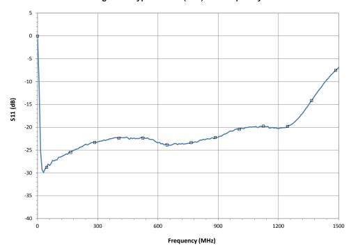
Figure 4: Typical Input Return Loss (S11) vs. Frequency
