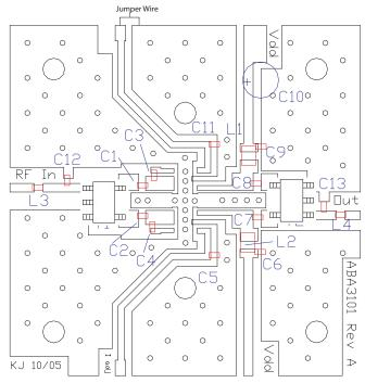
Figure 10: Evaluation Board Layout
