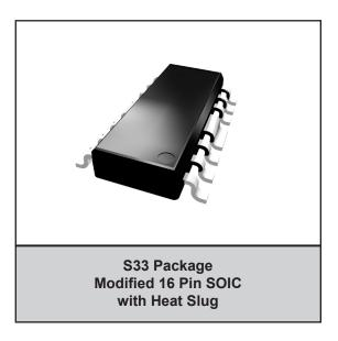
package with a heat slug, it is well suited for use in amplifiers where small size, reduced component count, and high reliability are important.
