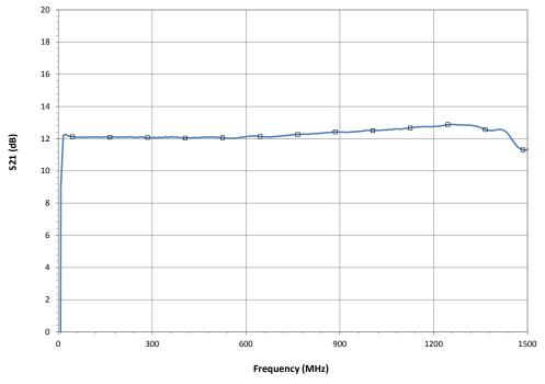
Figure 3: Typical Gain (S21) vs. Frequency
