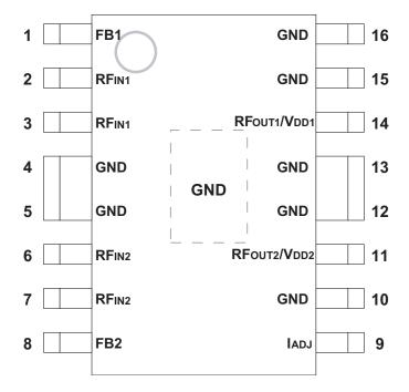
Figure 2: Pinout Diagram
