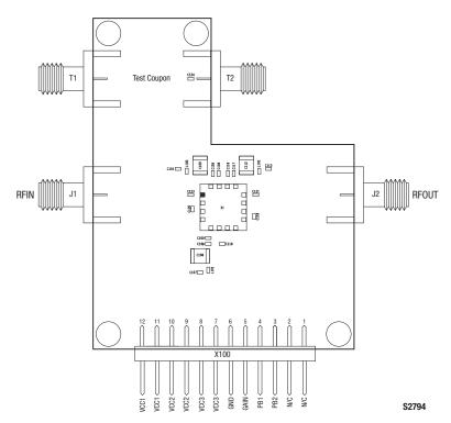
Figure 3. SKY65371-11 Evaluation Board Assembly Diagram
