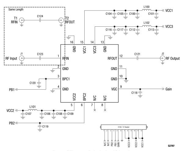
Figure 6. SKY65371-11 Evaluation Board Schematic
