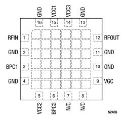
Figure 2. SKY65371-11 Pinout – 16-Pin MCM (Top View)
