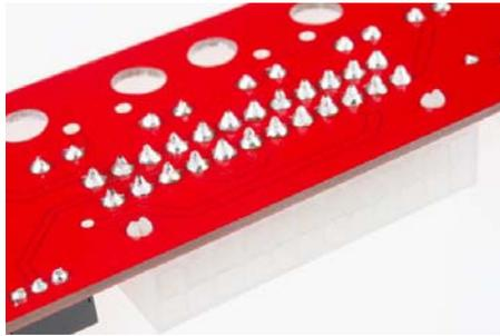
*Make sure you insert the ATX connector all the way into the board before soldering it down. The two white tabs should pop through the guide-holes.*
