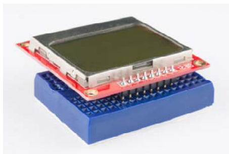
LCD with strait male headers soldered in, plugged into a mini blue breadboard.
