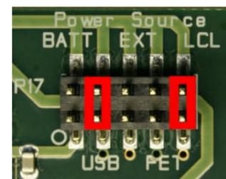
Depending on the power source, make sure you connect jumpers to the appropriate pins on the "Power Source" header. For operation of SmartRF Studio, it might be convenient to use the USB connection also for powering the board. Place the jumper such that pin 3-4 are shorted. A jumper should also be in position 9-10.
