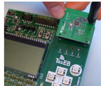
Insert the CC1175EM into a TrxEB. The connectors will only fit in one position so that the EM cannot be inserted the wrong way. Do not use excessive force on the EM. Remember to mount the antenna.
