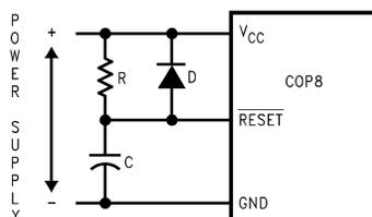
$RC > 5x$  power supply rise time or  $15 \mu\text{s}$ , whichever is greater.
