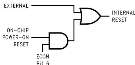
Figure 17. Reset Logic
