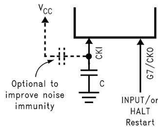
For operation at lower than maximum R/C oscillator frequency.
