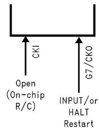
For operation at maximum R/C oscillator frequency.
