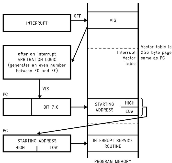
Figure 35. VIS Operation
