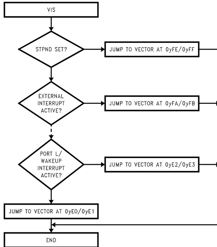
Figure 36. VIS Flowchart
