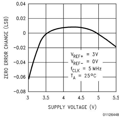
**Typical Performance Characteristics** (Note 9) The following curves apply for 12-bit + sign mode after auto-calibration unless otherwise specified. The performance for 8-bit + sign and “watchdog” modes is equal to or better than shown. (Continued)
