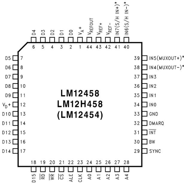
\* Pin names in ( ) apply to the obsolete LM12454 and LM12H454.
