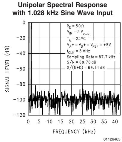
**Typical Dynamic Performance Characteristics** The following curves apply for 12-bit + sign mode after auto-calibration unless otherwise specified. (Continued)
