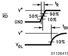
**FIGURE 9. TRI-STATE Test Circuits and Waveforms**
