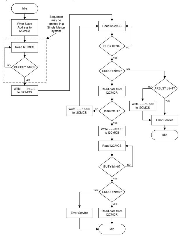
Figure 15-10. Master RECEIVE with Repeated START
