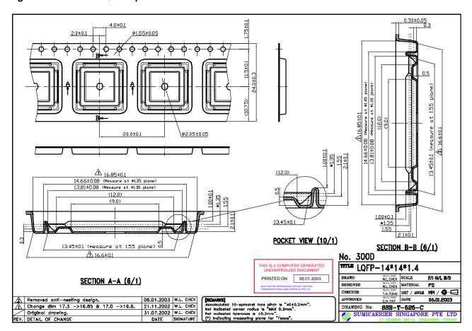
Figure C-3. 100-Pin LQFP Tape and Reel Dimensions
