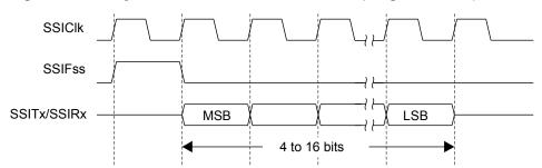
Figure 14-2. TI Synchronous Serial Frame Format (Single Transfer)
