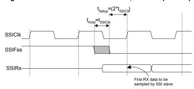
Figure 14-12. MICROWIRE Frame Format, SSIFss Input Setup and Hold Requirements
