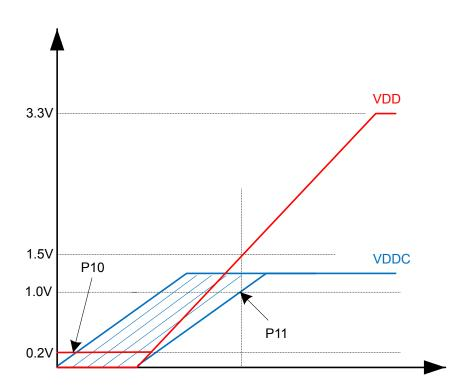
Figure 25-7. Voltage Requirements When Using an External  $\mathbf{V}_{\mathrm{DDC}}$  Source
