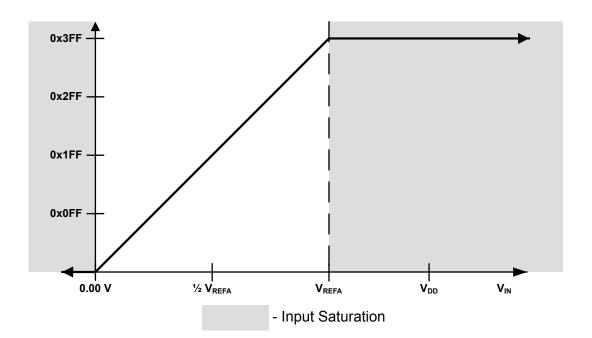
Figure 12-8. External Voltage Conversion Result
