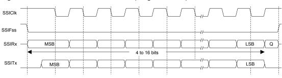
Figure 14-7. Freescale SPI Frame Format (Single Transfer) with SPO=1 and SPH=0
