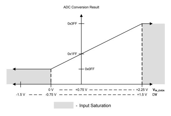
Figure 12-11. Differential Sampling Range,  $V_{IN\_ODD}$  = 2.25 V
