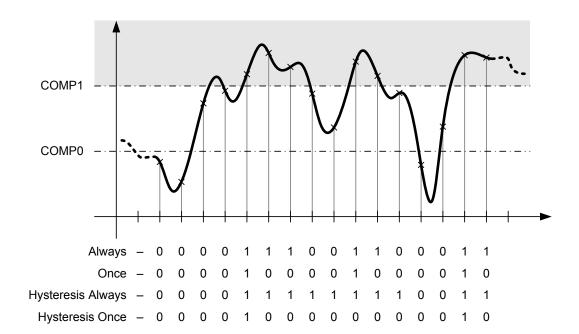
Figure 12-15. High-Band Operation (CIC=0x3 and/or CTC=0x3)
