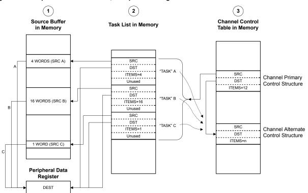
Figure 8-5. Peripheral Scatter-Gather, Setup and Configuration
