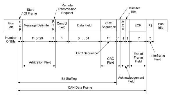
Figure 17-2. CAN Data/Remote Frame
