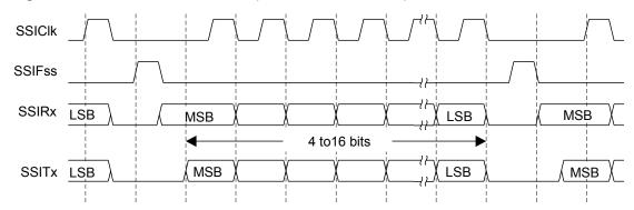
Figure 14-5. Freescale SPI Format (Continuous Transfer) with SPO=0 and SPH=0
