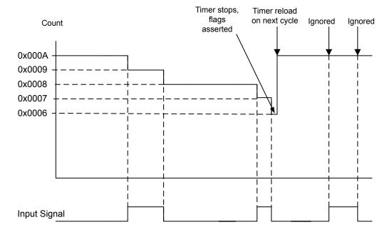
Figure 10-3. Input Edge-Count Mode Example
