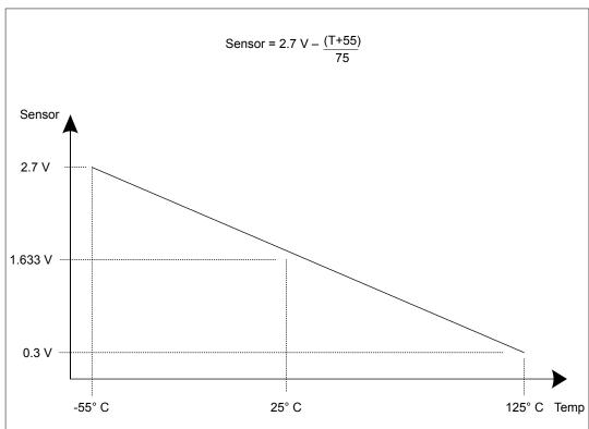
The temperature sensor reading can be sampled in a sample sequence by setting the  ${\tt TSn}$  bit in the **ADCSSCTLn** register. The temperature reading from the temperature sensor can also be given as a function of the ADC value. The following formula calculates temperature (in  ${\tt `C'}$ ) based on the ADC reading:
