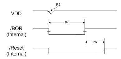
Figure 25-6. Power-On Reset and Voltage Parameters
