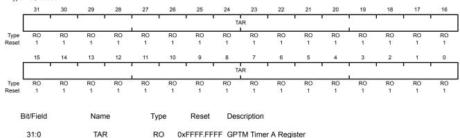
A read returns the current value of the **GPTM Timer A Count Register**, in all cases except for Input Edge Count and Time modes. In the Input Edge Count mode, this register contains the number of edges that have occurred. In the Input Edge Time mode, this register contains the time at which the last edge event took place.
