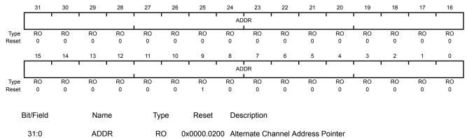
This field provides the base address of the alternate channel control structures.
