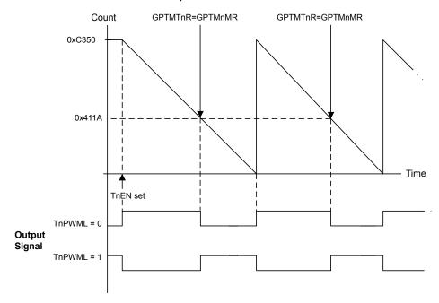
Figure 10-5. 16-Bit PWM Mode Example
