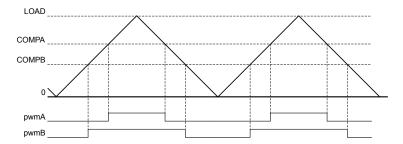
Figure 20-5. PWM Generation Example In Count-Up/Down Mode
