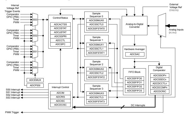
Figure 12-2. ADC Module Block Diagram
