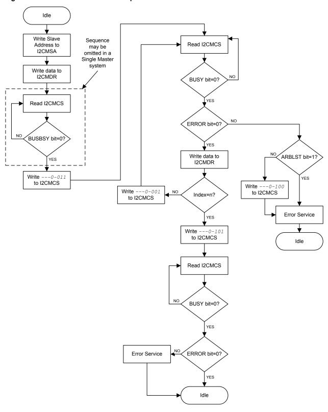
Figure 15-9. Master TRANSMIT with Repeated START
