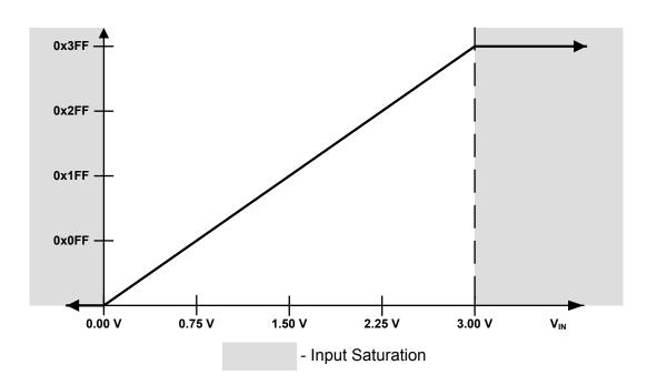
Figure 12-7. Internal Voltage Conversion Result
