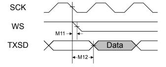
Figure 25-23. I<sup>2</sup>S Master Mode Receive Timing
