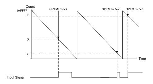
Figure 10-4. 16-Bit Input Edge-Time Mode Example
