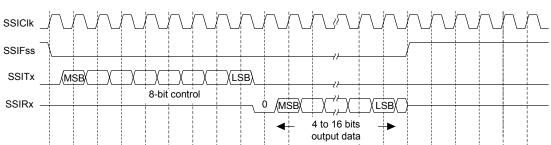
Figure 14-10. MICROWIRE Frame Format (Single Frame)
