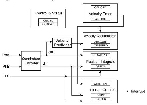
Figure 21-1. QEI Block Diagram
