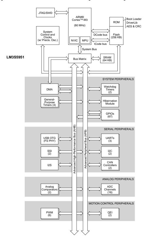
Figure 1-1. Stellaris LM3S5951 Microcontroller High-Level Block Diagram
