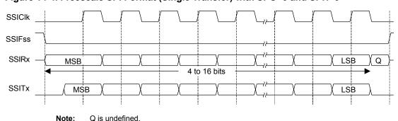
Figure 14-4. Freescale SPI Format (Single Transfer) with SPO=0 and SPH=0
