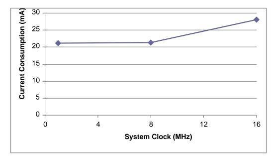
Figure 25-2 on page 1176 shows how typical current varies with frequency when using the PLL. Conditions are as follows:
