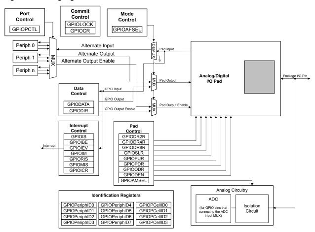
Figure 9-2. Analog/Digital I/O Pads
