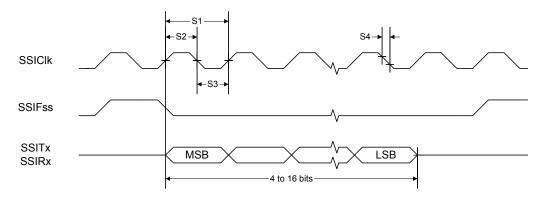
Figure 25-19. SSI Timing for MICROWIRE Frame Format (FRF=10), Single Transfer
