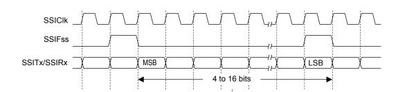
Figure 14-3. TI Synchronous Serial Frame Format (Continuous Transfer)
