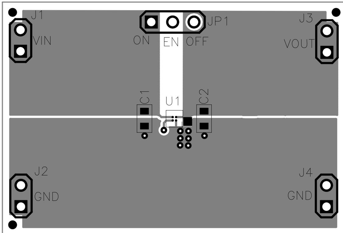
**Figure 3. Assembly Layer**
