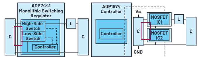
Figure 2. A monolithic switching regulator (left) and a solution with a controller IC (right), each with the geometrical arrangement of the hot loop.
