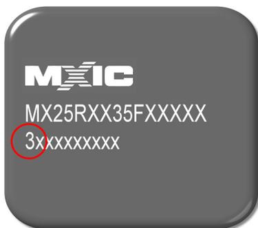
3). Package Label outside of shipping box can also identify the wafer Fabs for 2x3mm 8USON package. Lot# can be identified on the label. Lot# starts with number “2, 3, or 5” means the device is from Fab 2, whereas Lot# starts with number “7,8, or 9” means the device is from Fab 5 (see below marking illustration as an example, lot# starts with a “3” means it is from Fab 2)
