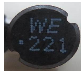
Marking with inkjet printing (with "WE" signature)
